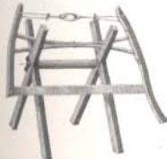
No. 3. Made of carefully selected Maple, well seasoned, natural finish. The legs are 2 inches \frac{1}{2} inch, 30 \frac{1}{2} inches long, strongly braced. The malleable iron castings at each side of the centre brace support the weight, making possible a light but durable Saw Bench. The centre brace is covered with a wood cylinder 2 x 14 inches. This cylinder revolves, and serves to protect the brace from the saw. When opened, the top of centre brace is 15 \frac{1}{2} inches from the ground. Price $4.25 per dozen
