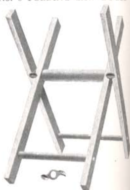
No. 3. Made of carefully selected Maple, well seasoned, natural finish. The legs are 2 inches \frac{1}{2} inch, 30 \frac{1}{2} inches long, strongly braced. The malleable iron castings at each side of the centre brace support the weight, making possible a light but durable Saw Bench. The centre brace is covered with a wood cylinder 2 x 14 inches. This cylinder revolves, and serves to protect the brace from the saw. When opened, the top of centre brace is 15 \frac{1}{2} inches from the ground. Price $4.25 per dozen
